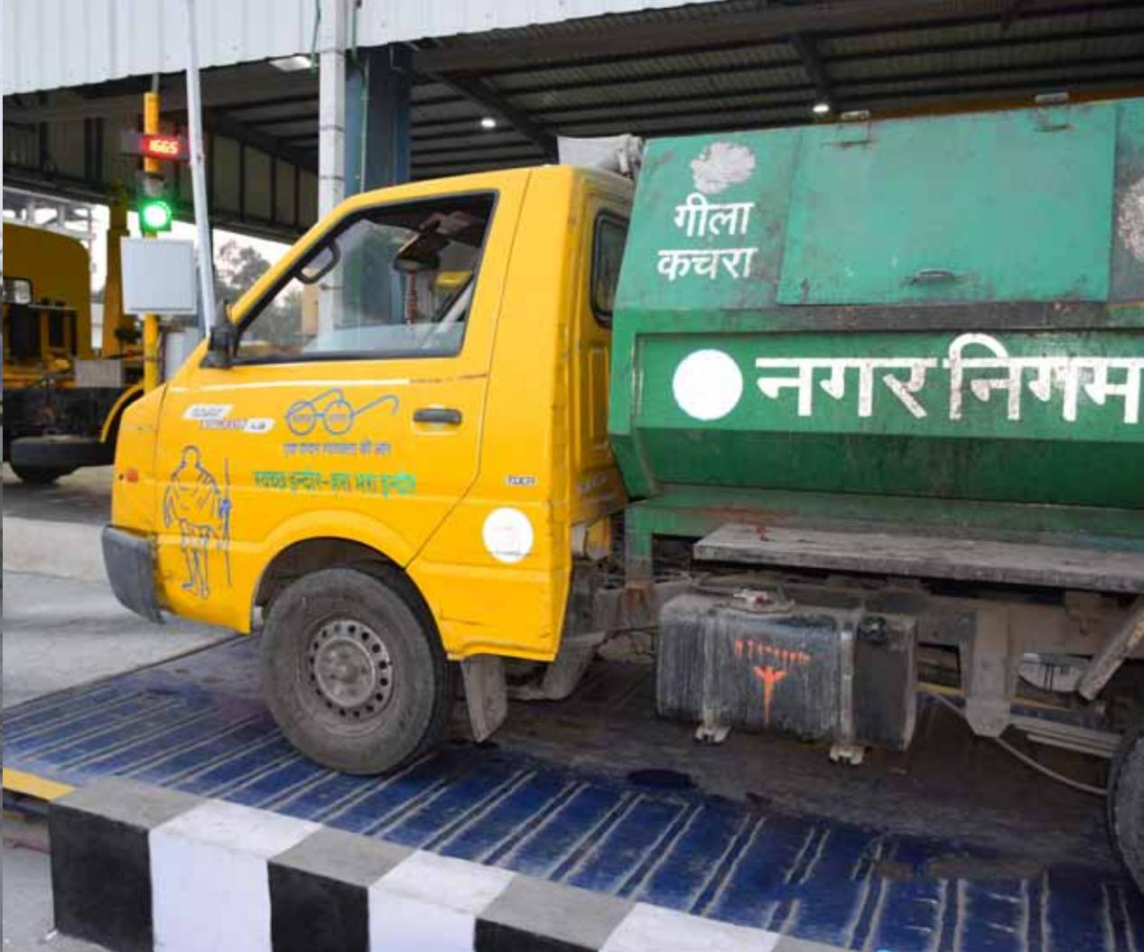
“Accurate weighing to know the quantity of wet and dry waste separately is the backbone of SWM. Automated man less weighbridges with RFID readers, automated boom barriers have been installed at all 10 transfer stations for temper proof system ”
